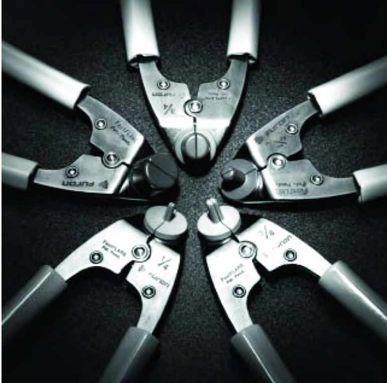
Furon FastFLARE forming tools are ideal for cold flaring PFA tubing. For use with Furon Flare Grip® and Flare Grip II PFA fittings.
