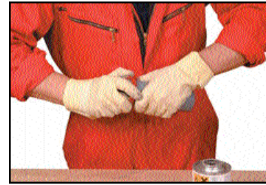
Chamfering the pipe
